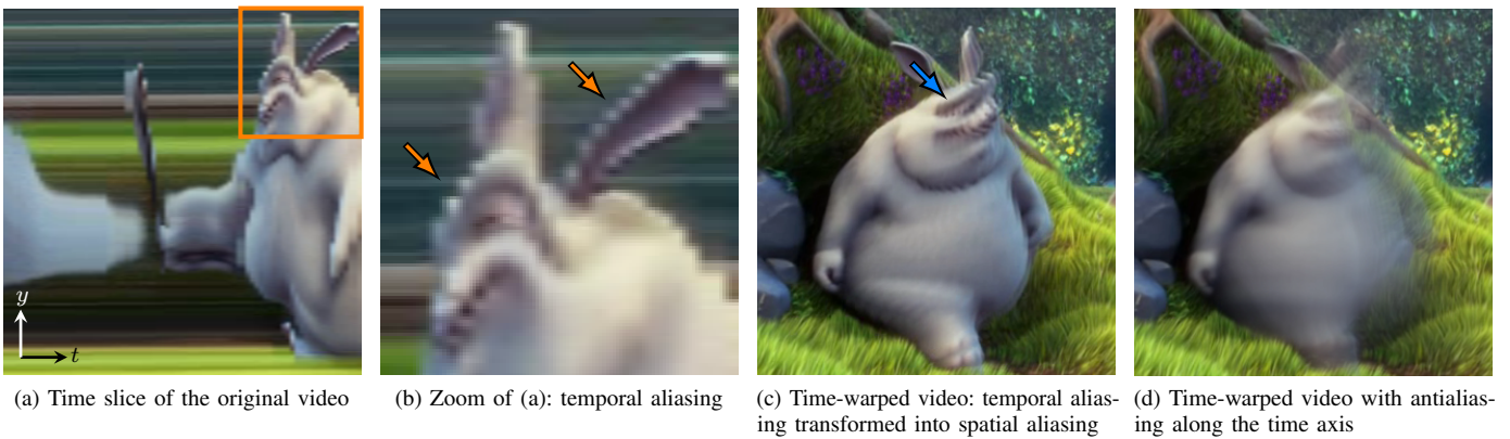
Fig. 13: (a) Time slice along the (y, t) plane of a video sequence containing object motion. (b) Zoom of (a), showing the presence of jagged edges, i.e. , temporal aliasing (orange arrows). (c) Time-warped video sequence, showing how temporal aliasing has been transformed into spatial aliasing (blue arrow). (d) Applying an antialiasing filter along the time axis removes aliasing artifacts but introduces motion blur. Deformation parameters: p_0 = (100, 100, 20) , f = (0, 0, 100) , \varepsilon = 60 .
