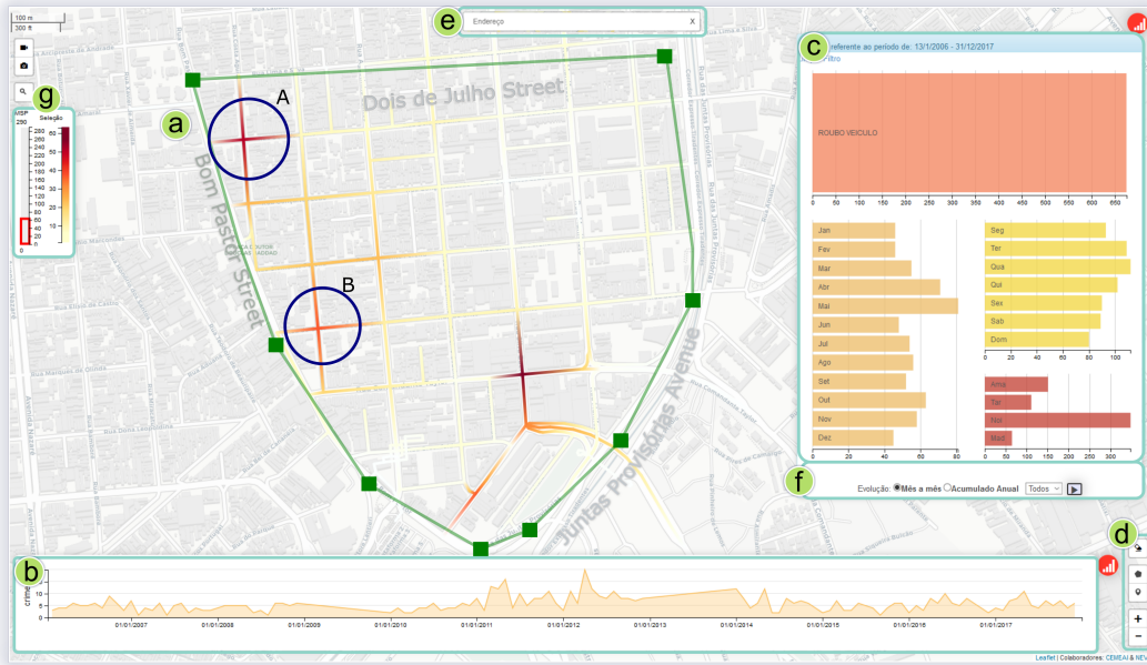
Fig. 2. An overview of the Mirante tool, a set of spatiotemporal visual resources enabling the exploration of crime patterns in a region: (a) Street-level Heatmap, (b) Temporal Evolution View, (c) Temporal Histogram View, (d) Selector toolbox, (e) Address Search Bar, (f) Evolution Animation Controller, and (g) Local/global crime ruler.
