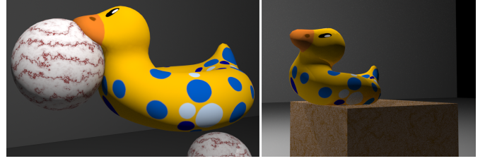
Fig. 3. Duck Lifebuoy (Bob) is simulated with St. Venant - Kirchhoff (left) and Neo - Hookean (right) materials and collision handling is tested. Left: Sphere collision constraint. Right: Convex objects collision constraint.
