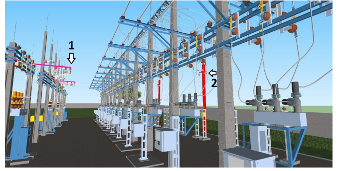
Fig. 11. Example image from the 3D model of the substation. Labels 1 and 2 indicate structures added to support the installation.
