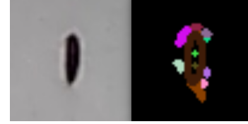
Fig. 17. Preprocessing done by PIA extractor - Sample with Failure (Hole).
