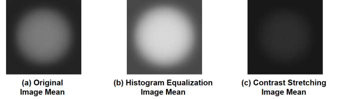
Fig. 4. Mean images of ICPR 2014 data set: (A) original, (B) after histogram equalization, and (C) after contrast stretching.
