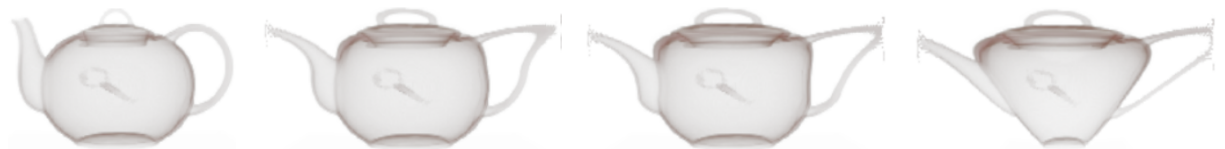
Fig. 13: In this example we show the taper deformation being applied in certain volume regions. The first figure is of the non deformed volume. The second one shows that only the upper half of the volume is being deformed. The third figure is of the volume with the deformation applied to 80% of its region. And the remaining figure shows the volume deformed in its totality.
