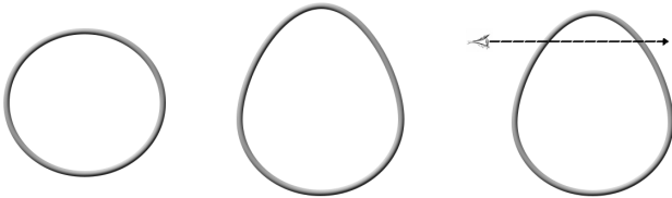
Fig. 3: Normal process of deformation of an object. First it is necessary to create the deformed object (middle) from the original (left) and only then run the ray casting (right).
