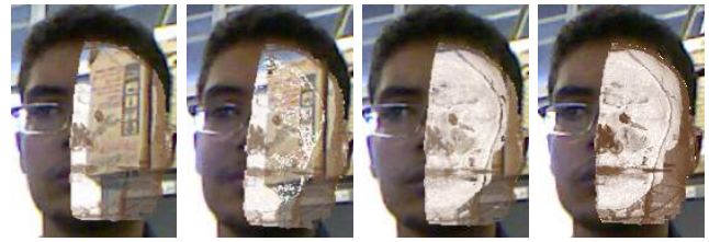
Fig. 6. F+C visualization based on visible background on CT data. By using an user-defined parameter, the medical volume can be rendered in different ways [12].
