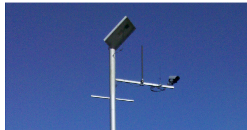
Fig. 3. Sensor node that acquired the images.
