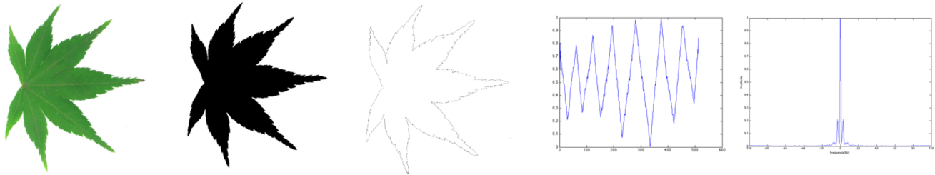
Fig. 1. Leaf shape modeling in the frequency domain. This figure shows the digital image process in combination with the Fourier descriptor for extracting a leaf shape signature. From left to right: original image; binary representation; extracted leaf contour; edge-centroid distance measure; normalised Fourier coefficients.
