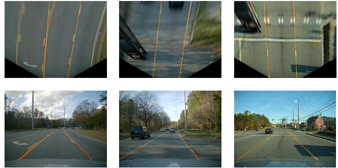
Fig. 16. Qualitative comparison: proposed system (red) and hough-based (yellow). From left to right, frames: 532 (S1C1), 144 (S2C2), and 565 (S3C1).
