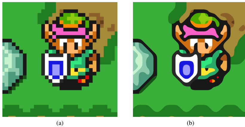
Fig. 19: The Legend of Zelda: A Link to the Past (SNES) frame scaled 16 times (a) nearest neighbor (b) our method (Original image ©Nintendo Co., Ltd)
