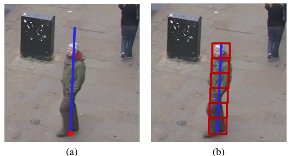
Fig. 1. Initialization procedure. (a) Selection of the foot point (red dot), and its vertical expansion (blue line). (b) Selection of the head point and patch creation (along a vertical line in the WCS).
