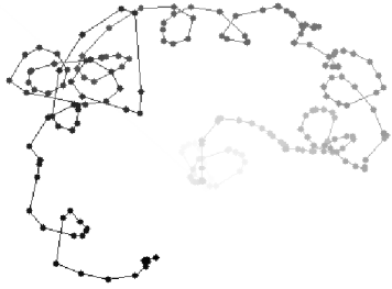
Fig. 2. Example of laser projection tracking along 255 frames. Darker lines and points show points indicated by the user more recently.
