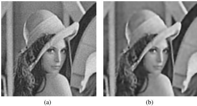
Fig. 8. (a) CGSR with \beta = 1 , \alpha = 0.125 ; (b) CGSR with adaptive constraints, \beta = 1 , \alpha = 0.125 and \mu = 100 .
