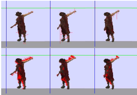
Figure 6. Comparison of the methods used to determine the 3D velocities. Top: Lucas-Kanade algorithm extended to 3D space. Bottom: Proposed method to perform the fusion of the 2D optical flow vectors in 3D space.
