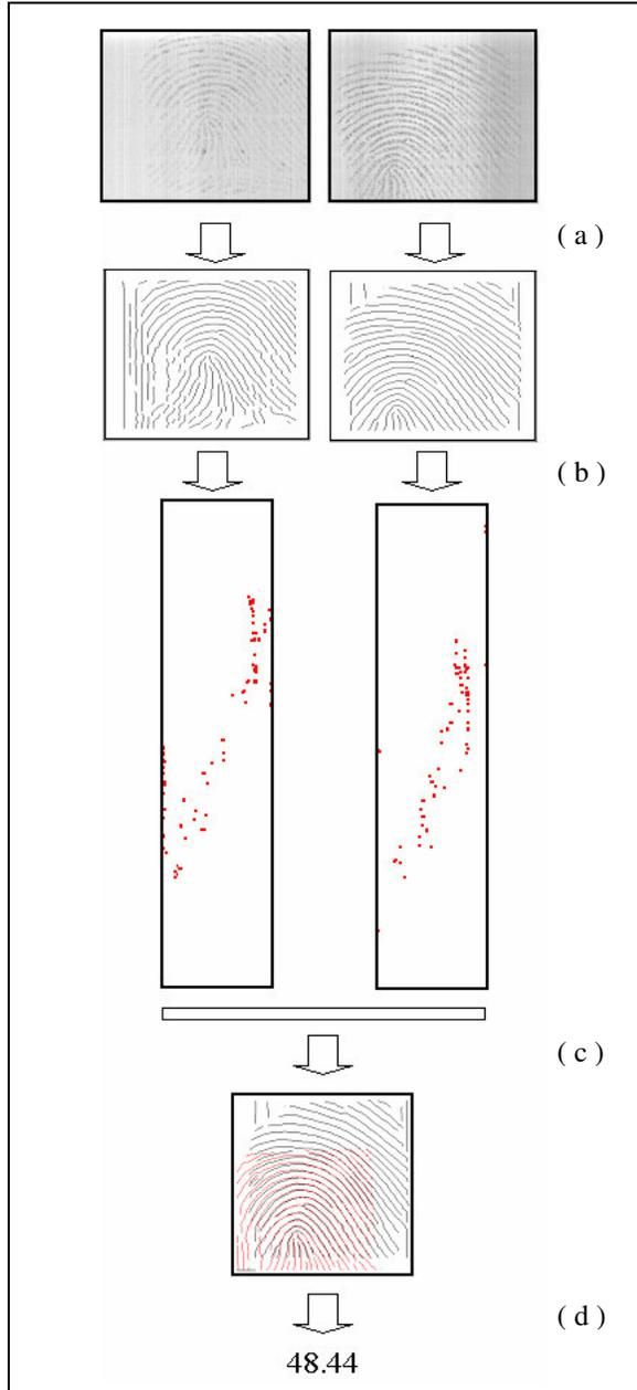
**Figure 1.** Major steps of the ridge-based matching technique. (a) Fingerprint ridges are detected and thinned; (b) Most significant Hough space peaks are detected; (c) The rotation and translation parameters for fingerprint registration are estimated from the two sets of peaks; (d) A correlation score is computed for the alignment.
