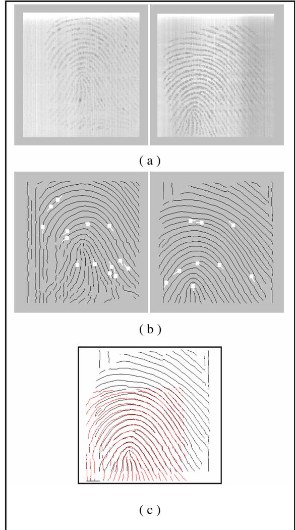
**Figure 9.** (a) A genuine fingerprint match rejected by the minutia-based matcher and correctly accepted by the ridge-based matcher; (b) Minutia points detected; (c) Alignment obtained by the ridge-based technique.
