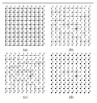
Figure 3. Segmentation by tree pruning. (a) A 4-connected graph representation of an image G with one seed pixel (bigger dot) inside the object. (b) An optimum-path forest for  $f_{peak}$ , with minimum path costs shown. (c) The number of descendants of each pixel in the forest. (d) Segmentation obtained by pruning the subtree of the pixel with 84 descendants. The numbers indicate object labels assigned to each pixel (0 for the background, 1 for the object).
