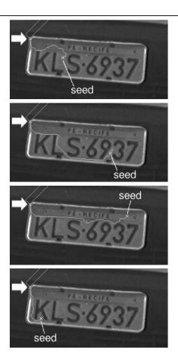
Figure 11. Segmentation of the same license plate with different seed locations: the automatically detected leaking point (indicated by the arrows) is always the same, since it is the stronger connection between the object and the background.
