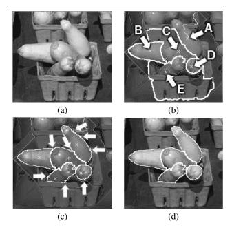
Figure 7. Multiple object segmentation by tree pruning. (a) An image of a basket with squashes. (b) Image with the number of descendants, after seed selection for each squash. (c) Result of a few prunings indicated by arrows. (d) Resulting segmentation.
