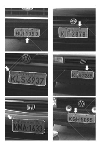
Figure 10. License plate segmentation by tree pruning. One seed is selected inside each plate, and the first pruning point detected automatically (indicated by the arrows) segments the plate.
