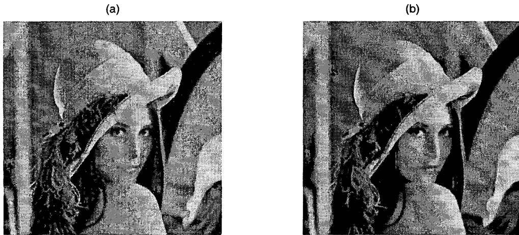
Figure 3: Noisy Lenna image filtered by: (a) wiener2 (PSNR = 28.71 dB); (b) our technique (PSNR = 30.02 dB).
