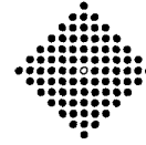
Figure 7: Diamond-shaped structuring element.
