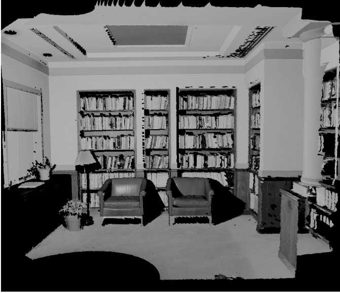
LEFT: Organized, noisy, massive range data set: 6.48 million points, 143858 points retained, 267131 triangles, 88.5 secs RIGHT: Notice the noise and the microfacets on the floor of the room
