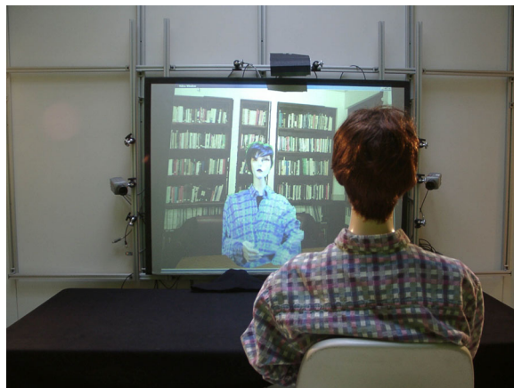
Figure 1: Our Personal 3D Video Teleconferencing Station. The system is displaying a synthesized view of the participant, acting as a 3D mirror (we do not yet have a second system to run in full-duplex mode).
