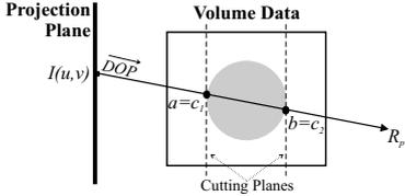
Figure 5: Cutting planes delimiting the sampling interval.
