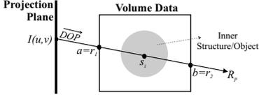
Figure 4: Sampling interval when no cutting tools are used.
