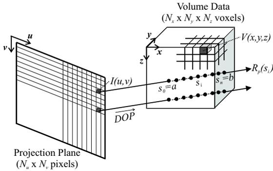
Figure 1: General scheme of a ray casting algorithm.
