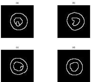
Figure 11: Watersheds computed for the tomographic image using the proposed denoising/enhancement technique with post-processing.
