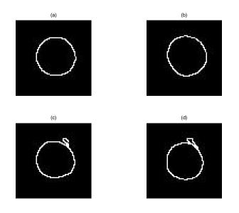
Figure 10: Watersheds computed for the tomographic image using the Prewitt operator to estimate the gradient image.
