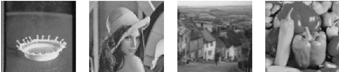
reconstruction scanning with steps of 8 pixels and using range blocks of 4x4 pixels
