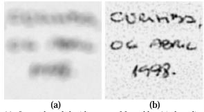
(a) Image degraded with an out-of-focus blur (circle radius equal to 15 pixels), with additive gaussian noise (variance = 16) (b) Restored image (ISNR=5.77 dB) by the Landweber iterative method with regularization and with inequality constraints (0 < f(i, j) < 240).
