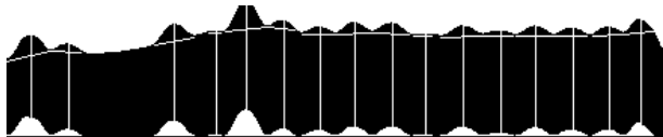
Figure 7: The results of maxima detection in the projection of the image shown in Figure 1, using Algorithm 3. The original projection was filtered with average filter. In this case, the lanes are correctly positioned in the image, despite of missing lanes. The tangent lines and the area above are also shown.
