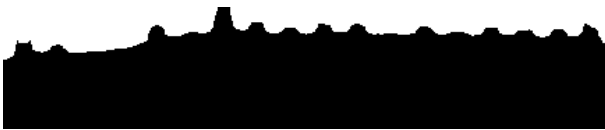
Figure 3: The projection of the image of Figure 2 onto x-axis, using sums.
