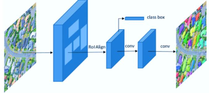
Fig. 3. Mask R-CNN neural network architecture, adapted of [33].
