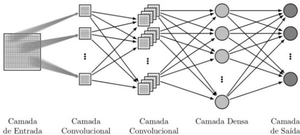
Fig. 2. EXAMPLE OF A CONVOLUTIONAL NEURAL NETWORK. Source [9]
