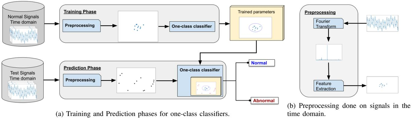
Fig. 3: Proposed fault detection process via one-class classification.
