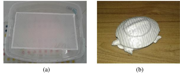
Fig. 1. A 3D printed object covered with carbon fiber pattern by a hydrographic printing technique. (a) Hydrographic film floating. (b) 3D printed object colored with hydrographics.
