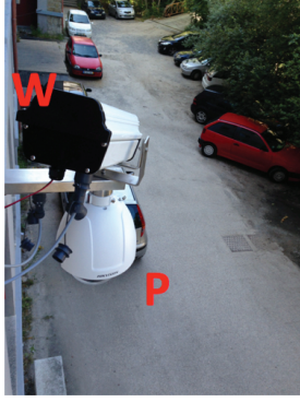
Fig. 2. Example of a synchronised pair of wide-view (W) and PTZ (P) cameras, from a master/slave laboratorial prototype mounted at the SOCIA: Soft Computing and Image Analysis laboratory outdoor wall. This prototype is able to automatically detect and track subjects passing by and acquire high resolution images of subjects heads located up to 50 meters away of the recognition system.
