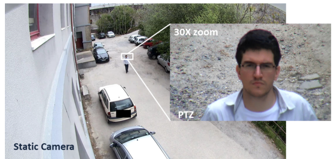
Fig. 1. Example of the data resulting from a master/slave dual camera architecture for biometric recognition in surveillance environments: while a wide view (static) camera covers the whole scene, the coordinates of detected human heads are sent to a calibrated Pan-Tilt-Zoom device that acquires data with enough resolution to be used in biometric recognition.
