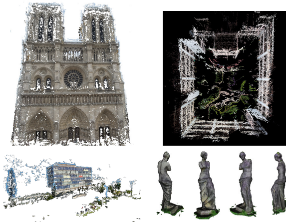
Fig. 5. Dense models estimated for the terrestrial datasets. In clockwise order from the top-left to bottom-right: notre_dame, ICEx_square, UFMG_rectory and UFMG_statue. All the last three datasets were estimated in less than 30 minutes with our approach.
