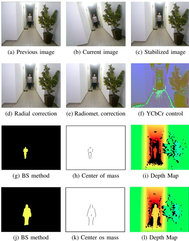
Fig. 3. Preprocessing System and Dynamic Objects System
