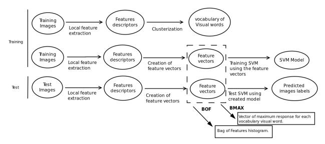
Fig. 1. Flowchart of BMAX and BOF algorithms.
