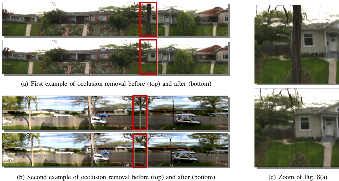
Fig. 8. Two examples where brushing has been used to remove occlusions. The regions of modification are shown in the red boxes.
