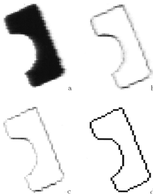
Figure 4: Original image of toy block (a), gradient image (b), first border (c) and second border (d)
