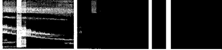
Figure 6: Flash video detection. Visual rhythm (left), white top by reconstruction (middle) and flash detected (right).
