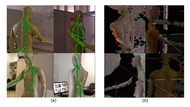
Fig. 5. Cross-talk interference among the RGB-D cameras. (a) deformed skeleton with wrongly placed joint position, and (b) pervasive holes in a point cloud reconstruction.
