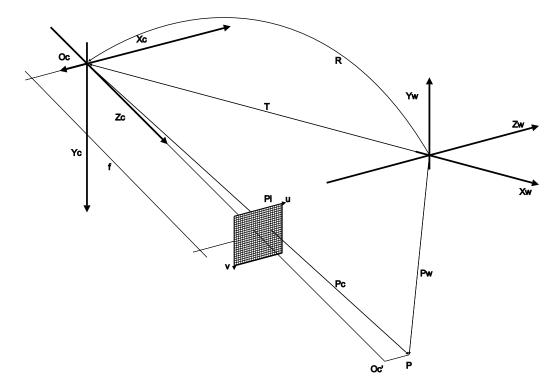
Fig. 2. Pin-hole camera model.
