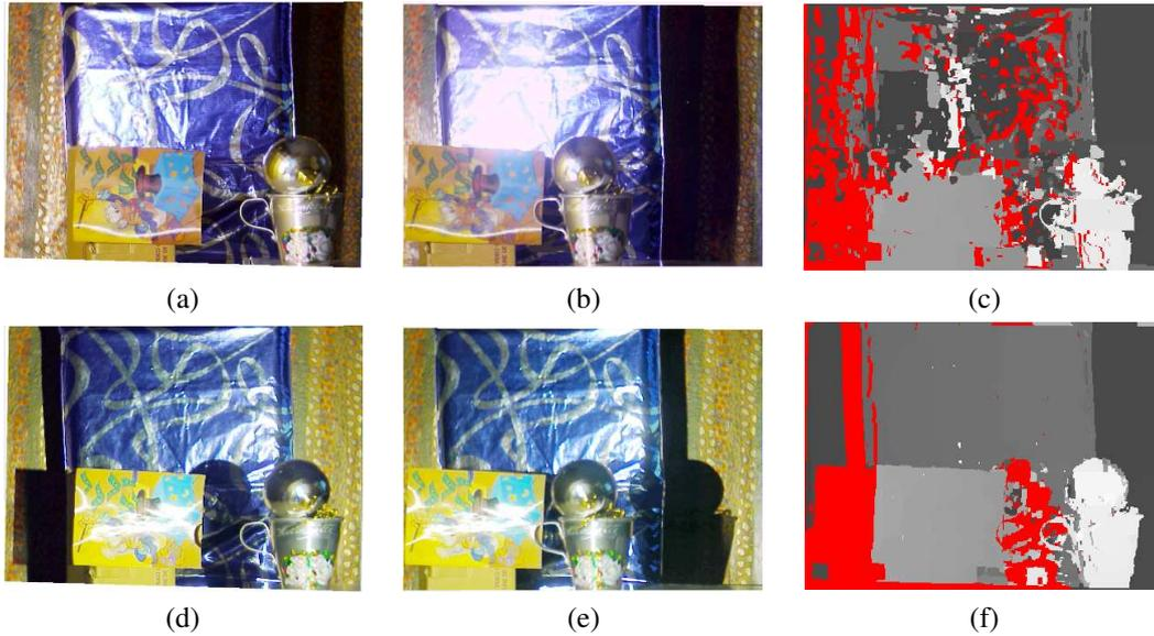
**Figure 11. Reconstruction of a more challenging scene: (a) and (b) stereo pair acquired under fixed illumination; (c) left-view depth map generated by conventional stereo, with half-occlusions shown in red; (d) and (e) stereo pair acquired with the proposed opto-mechanical system; (f) left-view depth map and occlusions detected by reciprocal stereo.**
