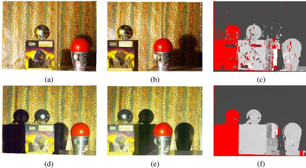
**Figure 12. Reconstruction of an even more challenging scene: (a) and (b) stereo pair acquired under fixed illumination; (c) left-view depth map generated by conventional stereo, with half-occlusions shown in red; (d) and (e) stereo pair acquired with the proposed opto-mechanical system; (f) left-view depth map and occlusions detected by reciprocal stereo.**
