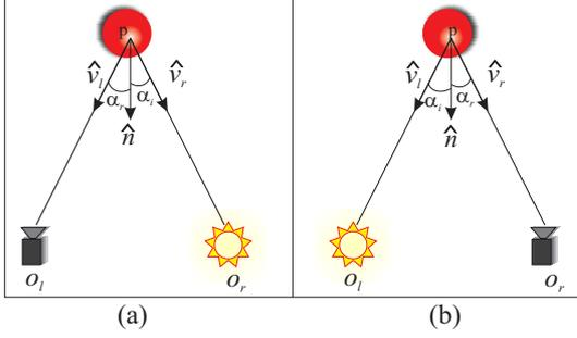
**Figure 1. Reciprocal stereo pair acquisition.** (a) An image is acquired by a camera at position  $o_l$ , and the scene is illuminated by a single source light at position  $o_r$ . (b) Camera and light source positions are swapped and a new image is acquired.
