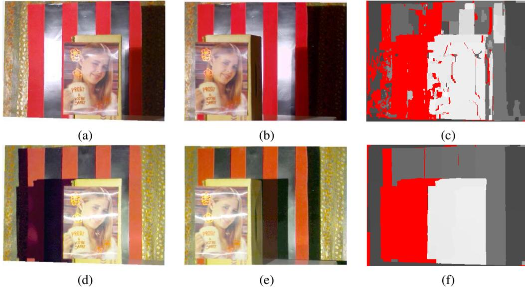
**Figure 10. Comparison between typical conventional stereo and reciprocal stereo results: (a) and (b) stereo pair acquired under fixed illumination; (c) left-view depth map generated by conventional stereo, with half-occlusions shown in red; (d) and (e) stereo pair acquired with the proposed opto-mechanical system; (f) left-view depth map and occlusions detected by reciprocal stereo.**
