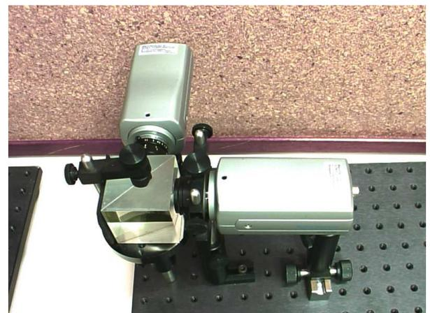
**Figure 9. System configuration used in the camera/light module calibration.**
