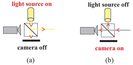
**Figure 4. One light/camera pair of the acquisition system. When the light source is on, the camera must be off and vice-versa. The beam-splitters have the role of making the light emission center and the camera projection center optically coincident.**
