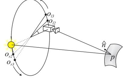
**Figure 2. Reciprocal pairs acquisition system** in which camera and light source are placed in diametrically opposite positions on a wheel. The reciprocal pair acquisition involves a rotation of the wheel by  $180^\circ$  after each image acquisition.
