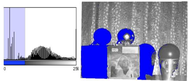
**Figure 6. Analysis of intensity histogram for shadow detection. Right: only intensities in the range highlighted in blue are regarded as possible shadow intensities. Left: only pixels in highlighted regions are regarded as being possible shadows.**
