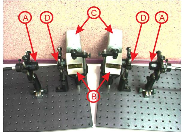
**Figure 8. The reciprocal pair acquisition system. We used two approximately collimated light sources (A); two beam-splitters (B); two CCD cameras (C); and two 16mm lens (D).**
