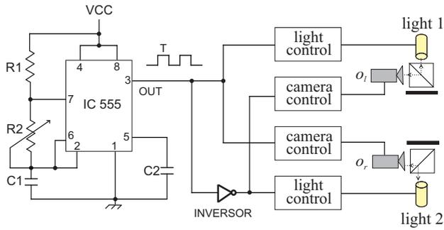
**Figure 7. Automatic system to acquire reciprocal video. It uses an oscillator circuit to guarantee the synchronism between the on/off control circuits of cameras and lights, within the optical system of the Figure 8.**
