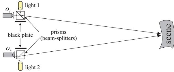
**Figure 3. The proposed reciprocal pair acquisition system. We use two cameras (at  $o_l$  and  $o_r$  positions), two light sources and two beam-splitters.**
