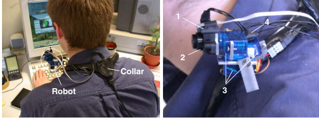
Figure 1. Wearable Visual Robot: (1) 2-axis accelerometer, (2) CMOS colour camera, (3) three motorised axes, (4) wireless video transmitter. The wearable interface box containing the data transceiver, micro-controllers and batteries is worn at the hip.
