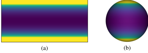
Fig. 2. Ideal dilation rates that should be adjusted depending on the latitude: blueish colors represent small dilation rates (not smaller than 1) while yellowish colors represent large dilation rates (in the limit case, infinity).
