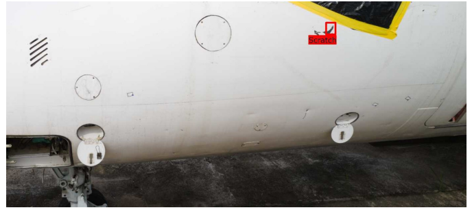
Fig. 1. Photo the side of an aircraft with defect detection result from the trained CNN. The detected scratch is marked with a red box on the upper right corner of the photo.
