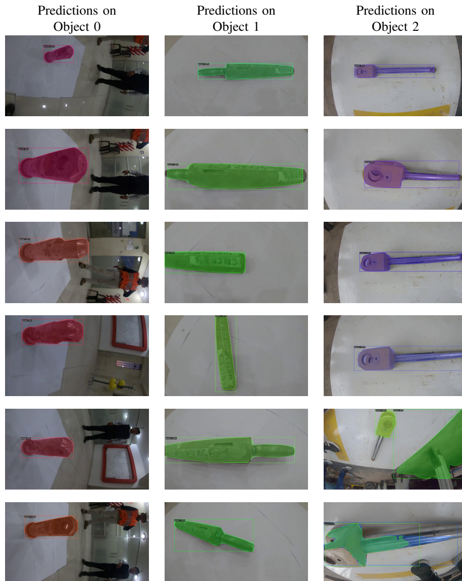
Fig. 6. Predictions on real data without Gaussian Blur of a model trained with synthetic data with Gaussian Blur (7 x 7). The last 2 rows of predictions on object 2 show some cases where the detection and segmentation fail.
