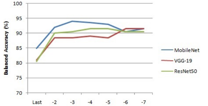
Fig. 4. LSVM balanced accuracy in last seven layers. MobileNet has better performance (94% in layer -3) and stays on top (layers -2 to -5). However, ResNet50 is more consistent (90% to 91, 5% from layers -2 to -7). VGG-19 has a growing accuracy from softmax layer into hidden layers.
