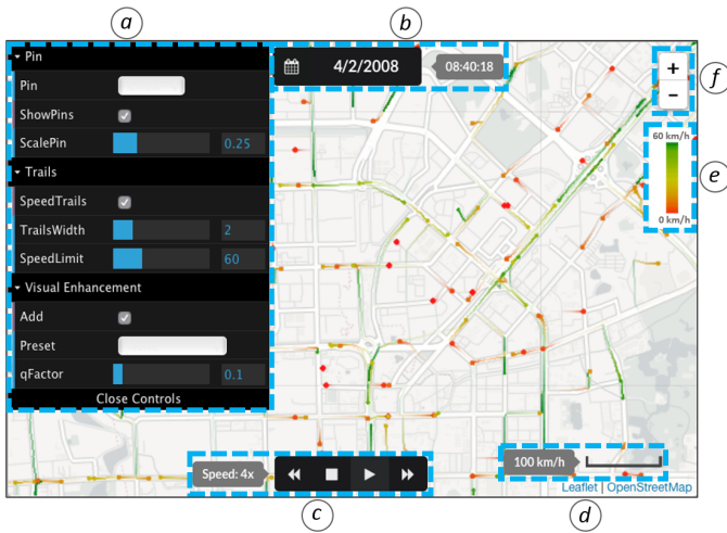
Fig. 1. Screenshot of a visualization of the traffic flow from 1,811 taxis moving at the same time. The image depicts the main functionalities of our developed tool such as the customization panel (a), where the user can set the marker size, speed limit, trail width, visual enhancement, and other parameters; the date and time display (b); the time control (c); the trail speed’s scale (d) and color encoding (e); and zoom control (f). A video showing the animated visualization is available on https://youtu.be/uyepCRSPyLo .
