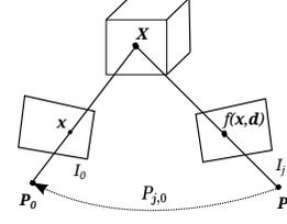
Figure 3. The reprojection function  $f(\mathbf{x}, \mathbf{d})$  establishes the correspondence between the pixels in  $I_0$  and  $I_j$  based on the depth information at the reference frame.
