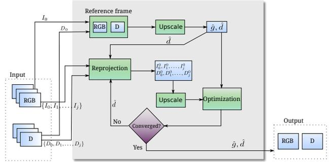
Figure 2. The main steps of the super-resolution methodology. First, all LR RGB-D images are reprojected to the reference frame and then an estimation of the super-resolution image  $\mathbf{g}$  and depth  $\mathbf{d}$  with the best reconstruction of the data is obtained in an iterative process.
