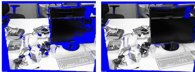
(a) Low Resolution Point Cloud (b) Super-Resolution Point Cloud
