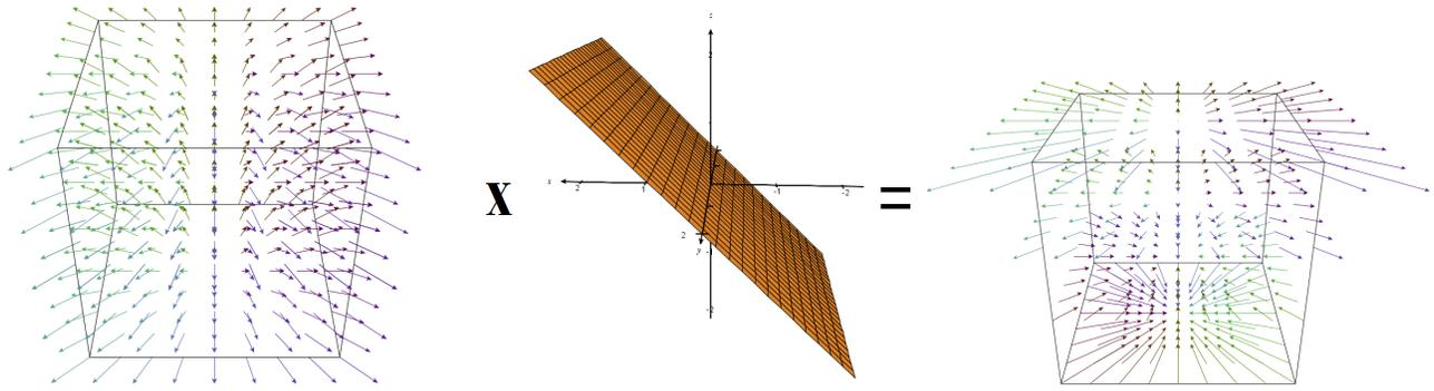
Fig. 5: By multiplying the expansion vector field  $\vec{v}(x, y, z) = (x, y, 0)$ , shown in the left image, by the function  $h(z) = z * k$  (middle image) we get the taper vector field that we can see in the right image.
