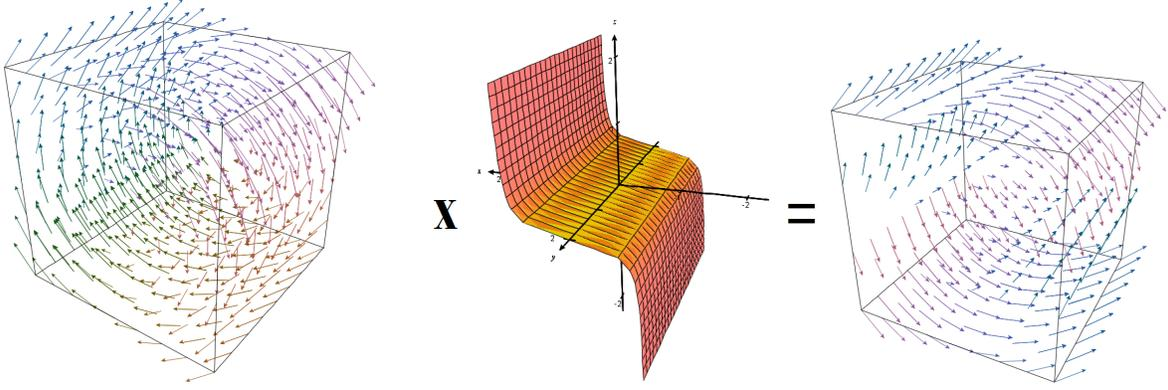
Fig. 7: A basic vector field representing a rotation around the x axis  $\vec{v}(x, y, z) = (0, -z, y)$  (left image) multiplied by the function  $h(z) = \arctan(10 * z) / (\pi/2)$  (middle image) creates the twist vector field (right image).
