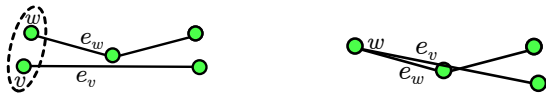
Fig. 17. The edges, e_w and e_v , cross each other after the vertices w and v are merged.
