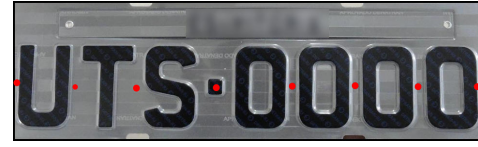
Fig. 2. Examples of the crop centroids on a license plate that feeds the PLS in the learning phase. The centroids are marked by the red points.
